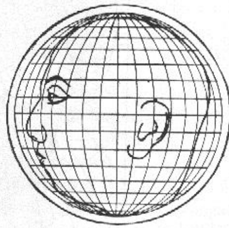
FIG. 44.—Man's head plotted on orthographic projection.
