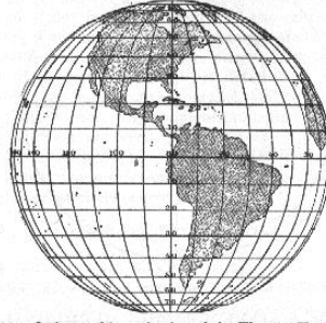
FIG. 34.—Orthographic projection of the Western Hemisphere.
